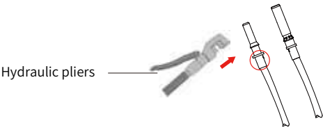
Pic 3.4 Crimp the contact pin to the wire
